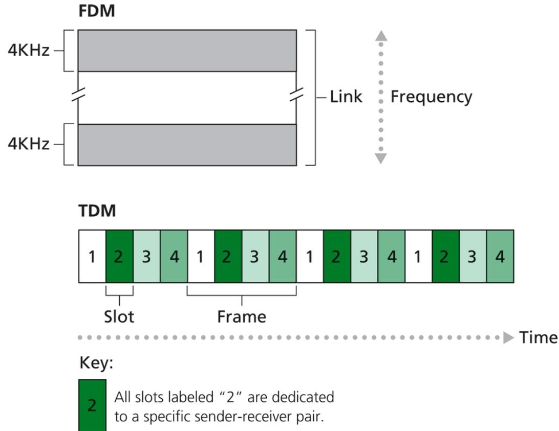
**Figure 1.6** ♦ With FDM, each circuit continuously gets a fraction of the bandwidth. With TDM, each circuit gets all of the bandwidth periodically during brief intervals of time (that is, during slots).
