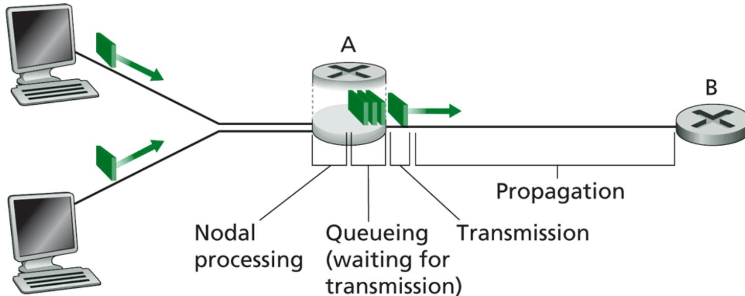
**Figure 1.13** ♦ The nodal delay at router A
